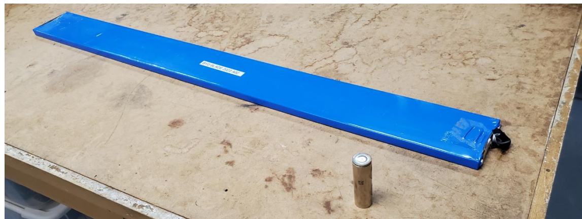
Figure 3.6 Comparison of Tesla Model 3 cell (cylindrical) and BYD Blade cell (large prismatic).
