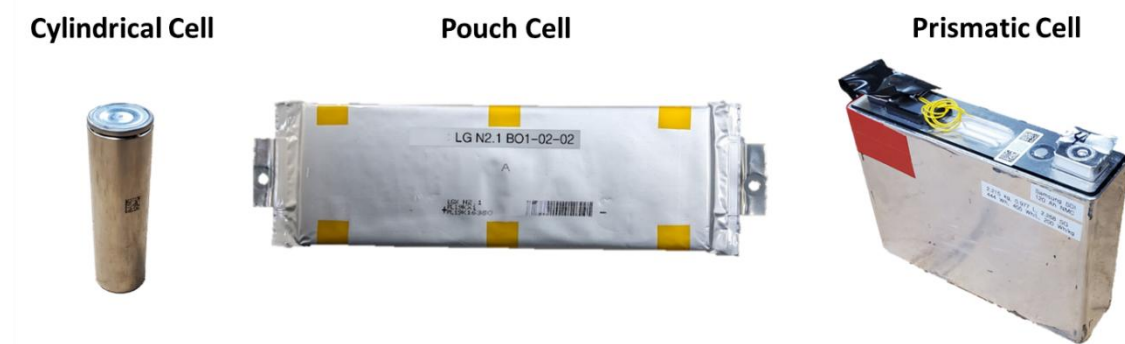
Figure 3.5 The three main lithium-ion cell formats: cylindrical, pouch, and prismatic.
